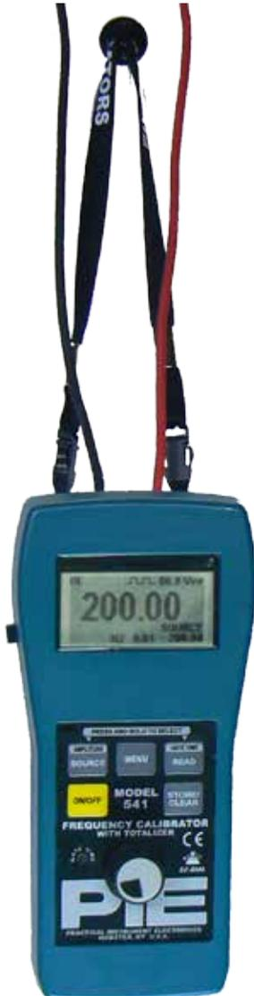
To suspend the calibrator from a pipe, conduit or rail release the connector from one side of the strap, pass the strap around the pipe, and snap the connector back into the strap.
