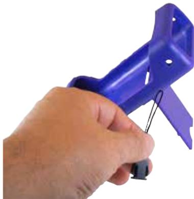
**1** Remove the PIE Calibrator from the boot and disconnect the two loops from the ends of the strap.
