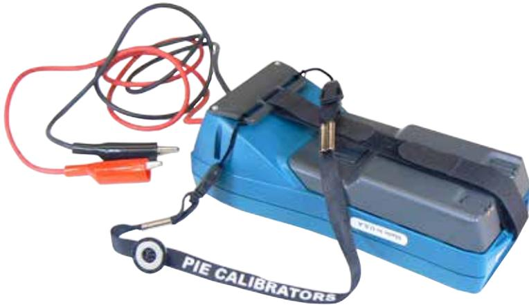
For the PIE Model 134 attach the loops of the strap to the belt clip on the back of the calibrator as shown below.
