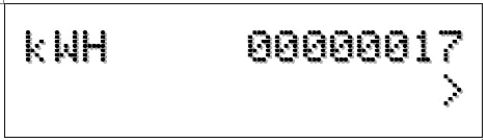
Fig. 13. The Class 1000 kWh meter displays readings in whole numbers, there are no decimals.
