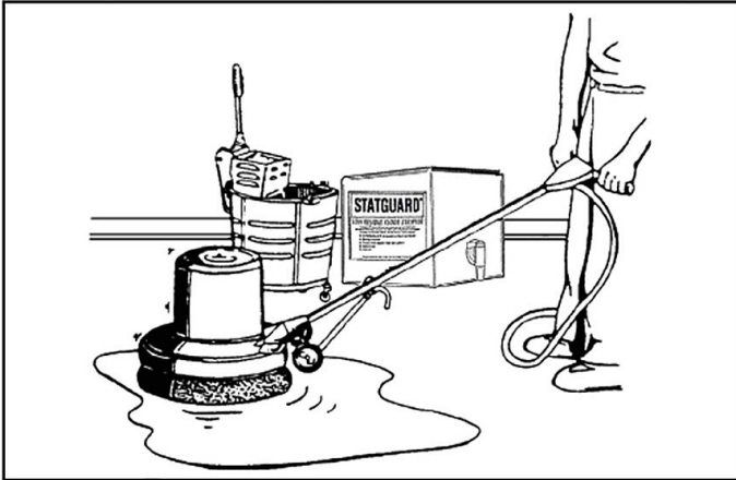
Figure 3. Stripping the floor
