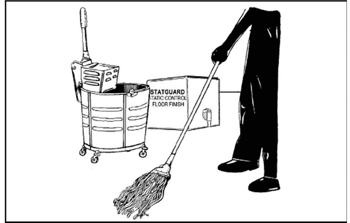
Figure 4. Applying floor finish
