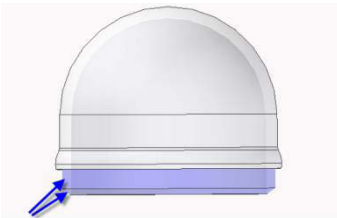
Fig. 49: Fitting the camera dome
