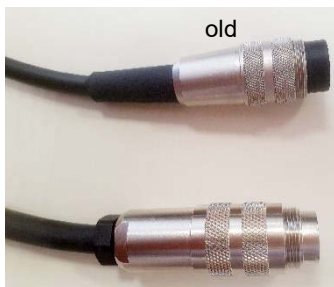
Fig. 9: Plug versions of the cable reel
