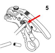
6. Grip the ends of a pair using the serrated teeth inside the front end of the tool (see red arrow in Fig 6)
