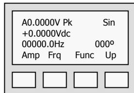
Pressing the button labeled FUNC starts the process of defining the desired output Waveshape (i.e., Sine, square, triangle, or sawtooth). See Page 11 for Function programming details.
