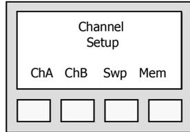
Pressing the button labeled ChA selects Channel A, and ChB selects Channel B. See Page 7 for Channel A programming details.
