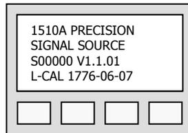
After about 10 seconds the display will change to the main Operator Entry Display.
