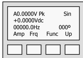
Pressing the button labeled Amp starts the process of selecting AC or DC output as well as VOLTS or Charge output. See Page 8 for Channel B Amplitude programming details.
