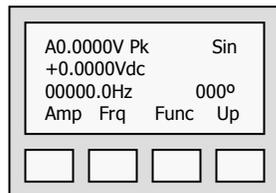
Pressing the button labeled FRQ starts the process of defining the desired output frequency in Hertz or RPM. See Page 10 for Frequency programming details.
