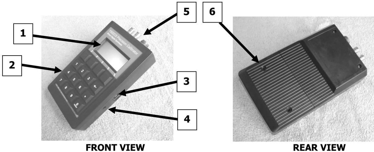
**1 - OPERATORS DISPLAY** – A 4 line by 18 character display displays current calibrator settings and is used during programming.
