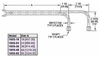
The **SERIES 160S** "S" Type Stainless Steel Pitot Tube is designed specifically for flow measurement of dirty, particulate laden air or gas streams typical in smoke stack and other environmental testing. Total and static pressure tubes are precisely aligned and welded together every 6 inches for maximum accuracy, strength, and long term durability. Permanent mount (PM) models include a 1" welded stainless steel sleeve and adjustable compression fitting with 1" MNPT mounting threads.
