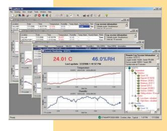
Customizable graphs in LogWare III with zooming capability are an easy way to analyze your data history, and data points that need to be explained can be highlighted, annotated, and referred to later. LogWare III statistics include min, max, spread, average, and standard deviation functions, and printed reports keep track of the number of temperature and humidity measurements that were found to be out of tolerance.
