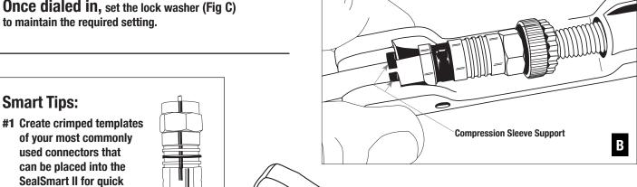
connector job. **#2** If connector is too long to fit into SealSmart II with adaptor head wide open, remove lock washer for additional space.
