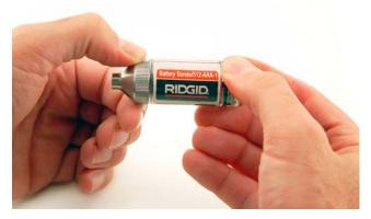
Turning the Transmitter ON and OFF – to turn the transmitter ON, tighten the battery cover fully, the LED will flash. To turn the transmitter OFF, loosen the battery cover <sup>3</sup>/<sub>4</sub> turn, the LED will turn off.
