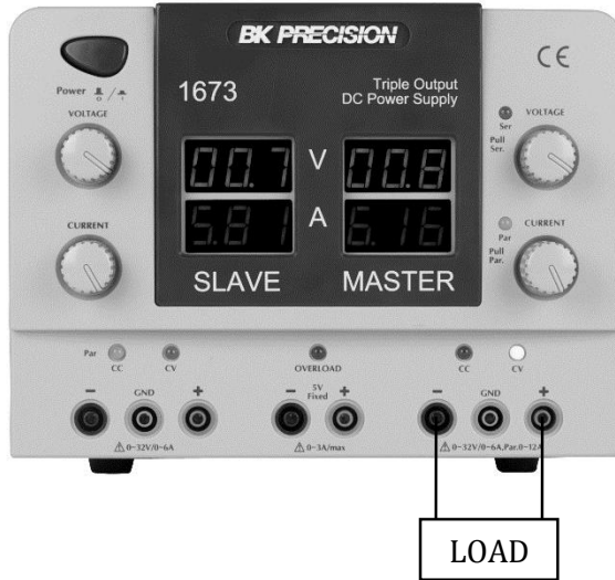
Figure 6 – Parallel Tracking Mode Load Connection
