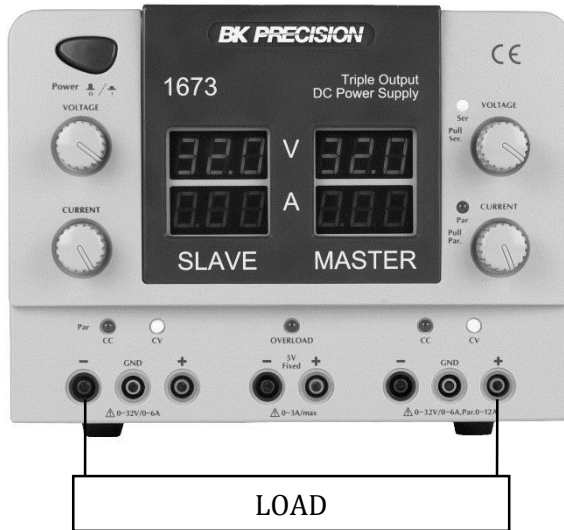
Figure 5 – Series Tracking Mode Load Connection
