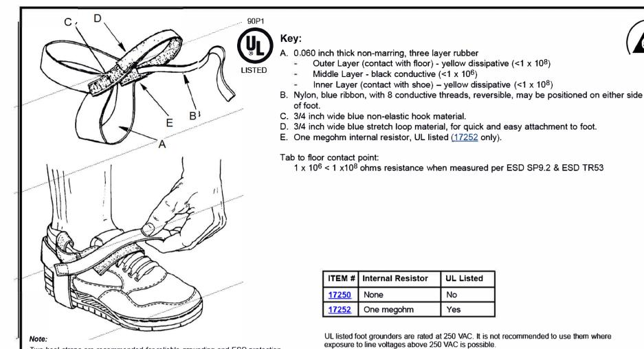
Two heel straps are recommended for reliable grounding and ESD protection, providing ground when one foot is off the floor.
