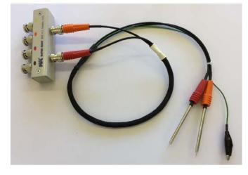
The 1905X Probe Kit allows the 1905A SMD Probe Leads to be used with Wayne Kerr analyzer models which do not have a 2-terminal setting for their front panel BNC connectors. This is achieved by using the 1023 4 into 2 BNC Adaptor. This kit is required when using 6500 or 4300 analyzers.
