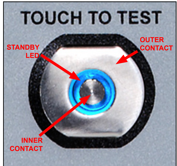
Figure 10. Steady-State Test Switch features and components
