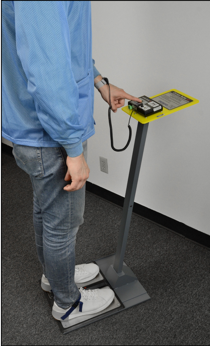
Figure 13. Using the 19271 Combo Tester X3 with Stand
