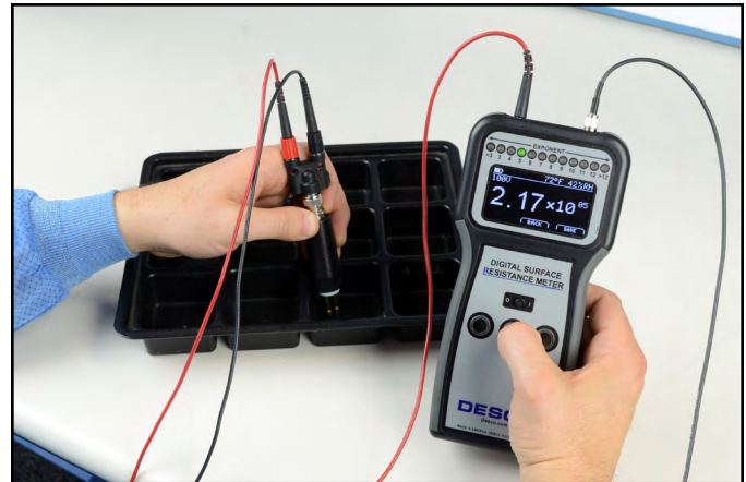
Figure 2. Using the Two-Point Resistance Probe with the Desco 19290 Digital Surface Resistance Meter
