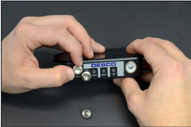
Figure 8. Installing the 10 mm snap adapters to the 19331 Full-Time Continuous Monitor
