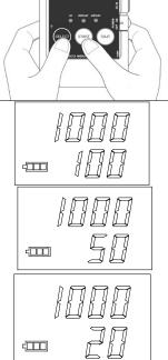
4. Point the plate in the airflow of the ionizer to be measured and press the START button.
