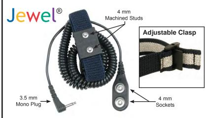
"If any part of the loop should open (become disconnected or have out of limit resistance), the circuit will go into the alarm state" [ref TR20.20], nonetheless, due to the redundancy inherent in the dual wire wrist strap design, the operator will continue to be grounded via the second intact wire.
