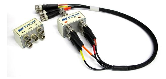
The 1J1001 4 to 1 BNC Converter is used to connect a Wayne Kerr 6500 analyzer to the Device Under Test using a single BNC connector. This is useful when the connection terminal of the DUT is a single BNC, such as some antennas. The outer of the single BNC is isolated.
