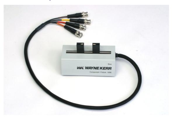
The 1006 Component Fixture is suitable for testing axial, radial and bandoliered components. The 4terminal connection to the Device Under Test allows a wide range of impedances to be measured accurately. The 1006 is recommended for maximum accuracy with conventional components due to its mechanical stability, and most Wayne Kerr accuracy charts specify the use of a 1006.
