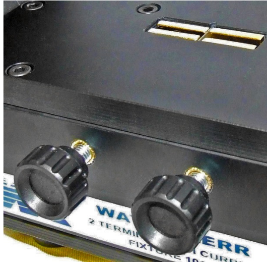
Device Under Test mounting location
