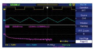
Display and measure the input signal's frequency spectrum. Select one of the 4 FFT windows: Rectangular, Hanning, Hamming, and Blackman. Use cursors to measure the spectral component's magnitude and frequency.
