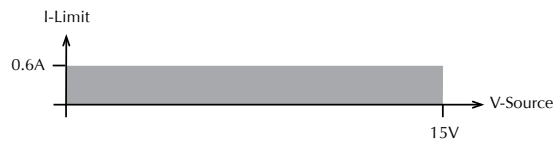
C) 500mA Measurement Range (Model 2303-PJ)
