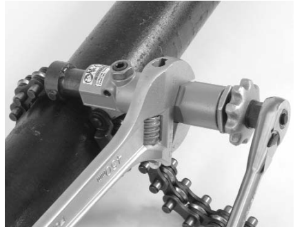
Figure 4 – Operating the Powered Soil Pipe Cutter – Manual Operation
