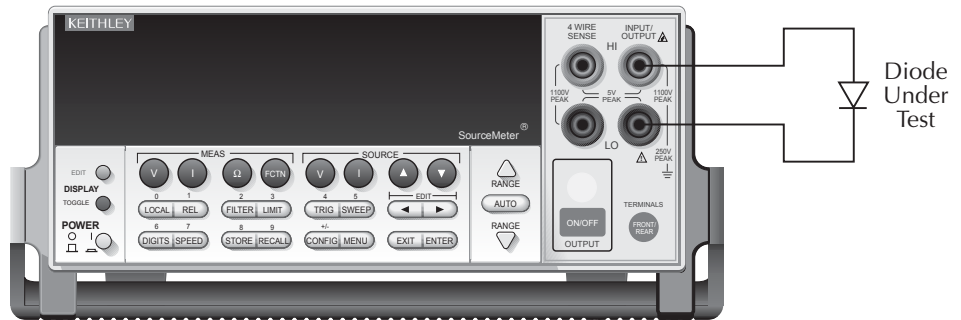
Figure 10-8 Connections for diode I-V tests
