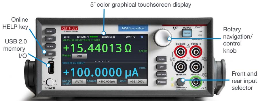
2450 front panel with high-resolution, capacitive touchscreen.
