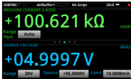
Figure 52: Resistance measurement using SVMI and reading ohms
