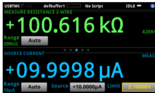
Figure 56: Resistance measurement using auto-ohms
