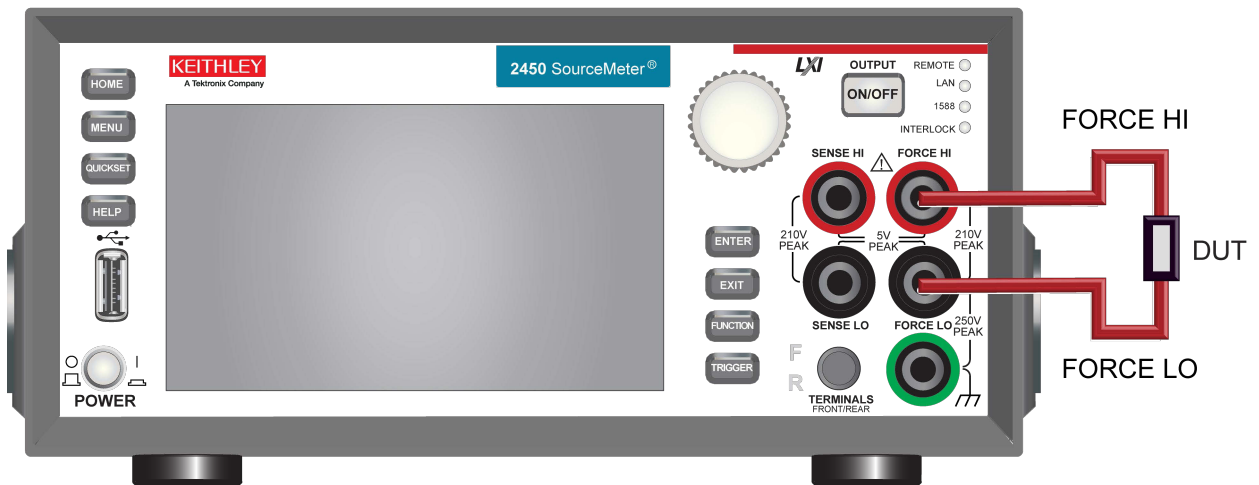
Figure 48: Two-wire DUT connections to the front panel
