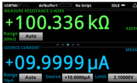
Figure 57: Resistance measurement autoohm
