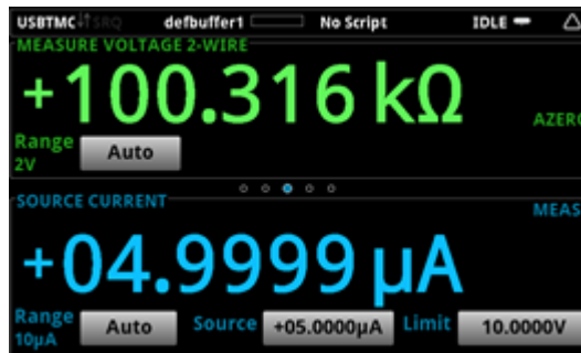
Figure 55: Resistance measurement SIMV and read ohms
