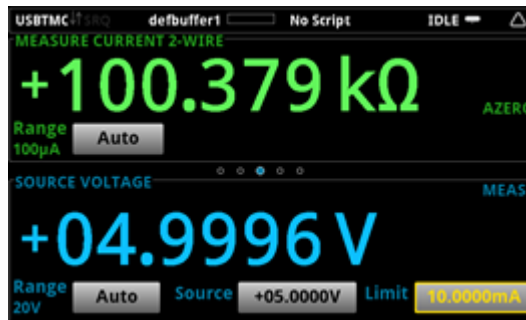
Figure 53: Resistance measurement SVMI and reading ohms
