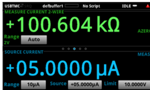
Figure 54: Resistance measurement SIMV SCPI example
