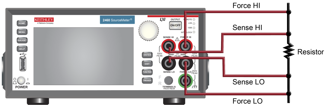
Figure 50: Model 2460 4-wire connections to the front panel
