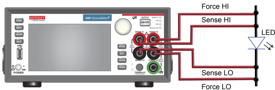
Figure 57: Model 2461 4-wire connections to the front panel
