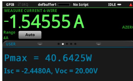
Figure 46: Solar panel I-V sweep results on the USER swipe screen
