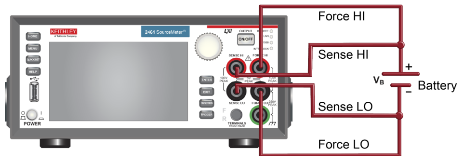
Figure 28: Front-panel connections for the battery discharge-charge application
