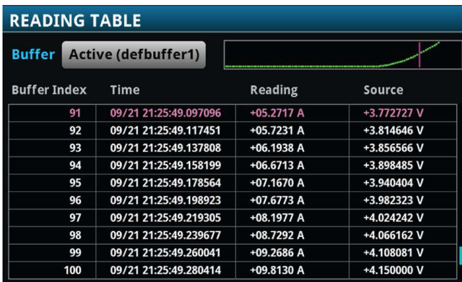
Figure 54: Reading table showing measurement results
