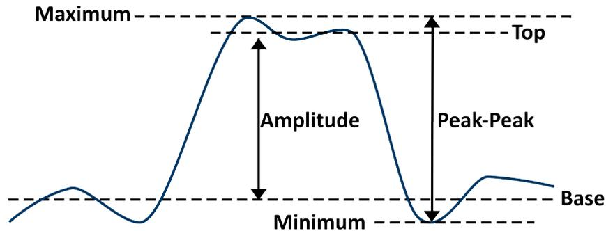
**Figure 10.2** Voltage Measurements
