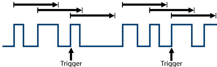
Figure 5.20 Interval Trigger
