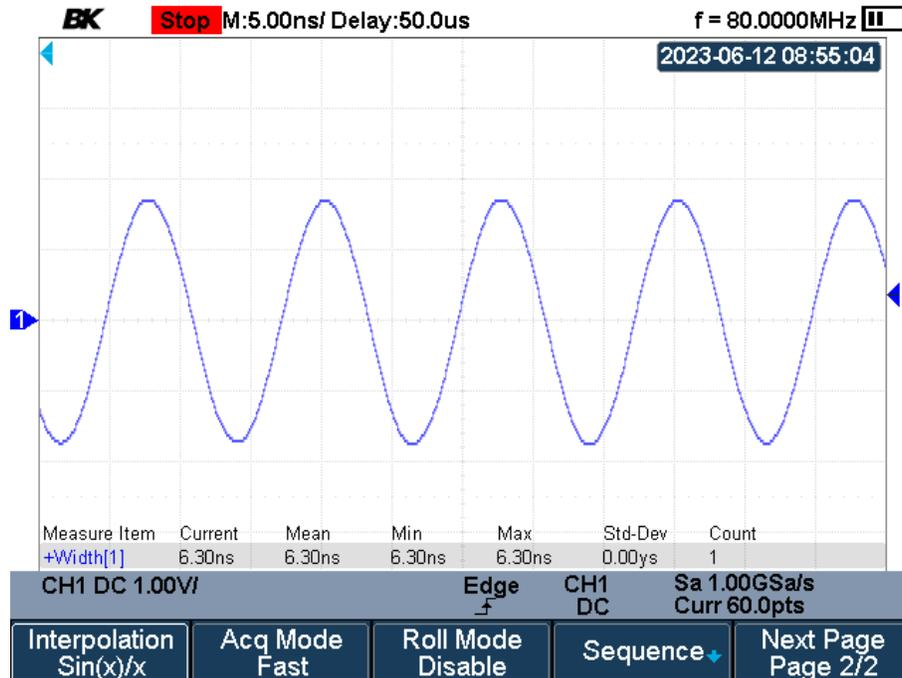
Figure 4.7 Interpolation Sin(x)/x
