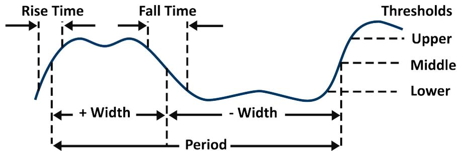
**Figure 10.4** Time Measurements
