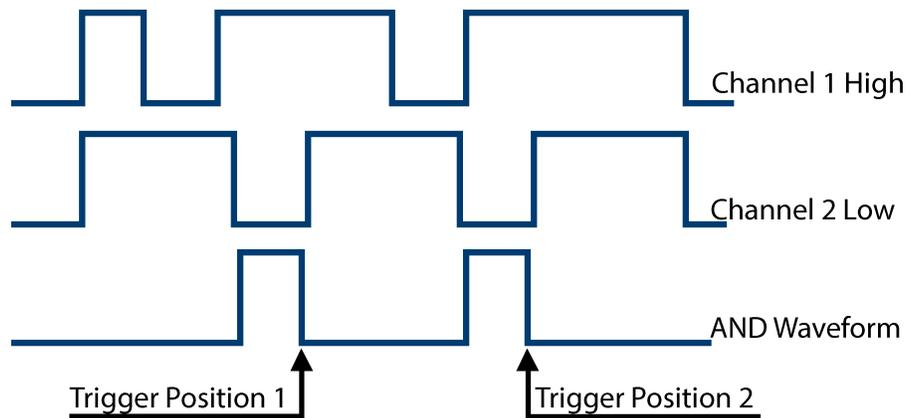
Figure 5.25 Pattern Trigger
