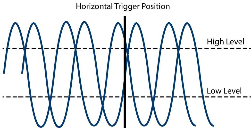
**Figure 5.19** Window Trigger
