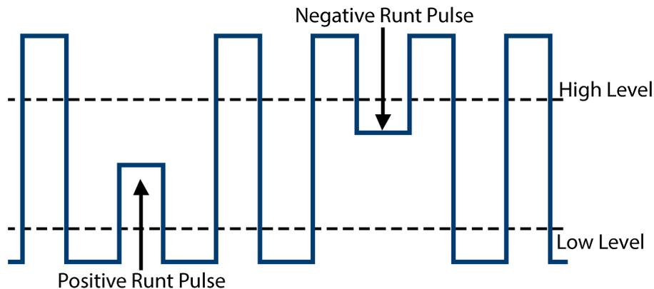
Figure 5.24 Runt Trigger
