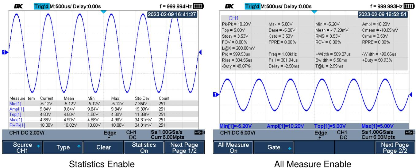
Figure 10.1 Measurements View
