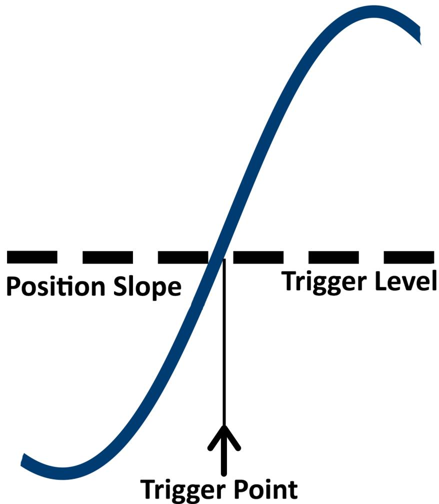
Figure 5.4 Trigger Point
