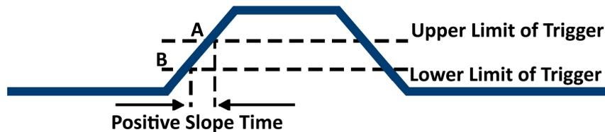
Figure 5.11 Slope Trigger
