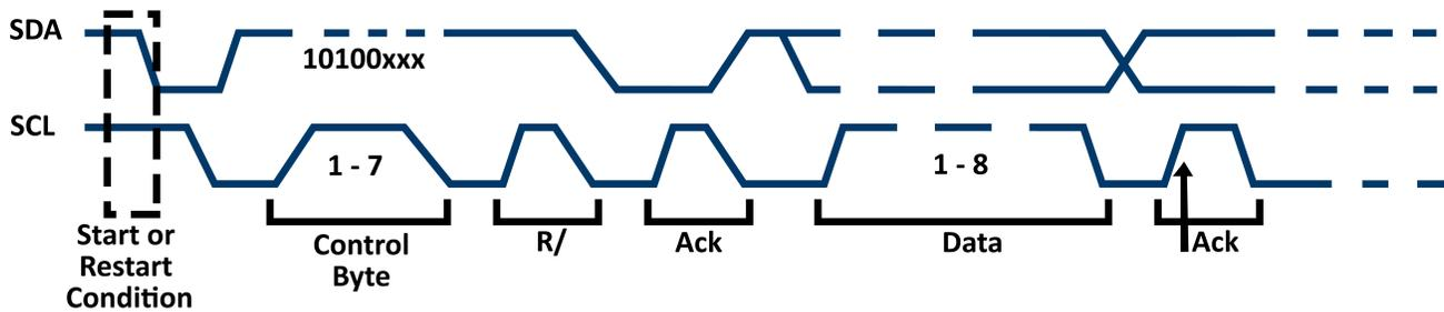
Figure 6.4 Restart, No Ack, and EEPROM Conditions
