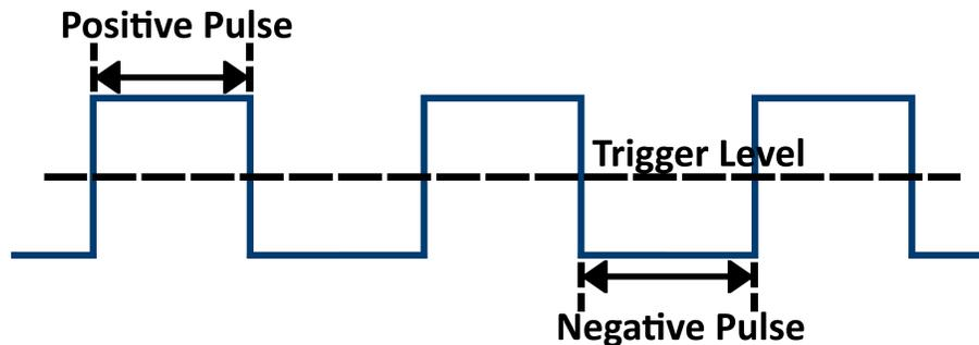
Figure 5.14 Pulse Trigger
