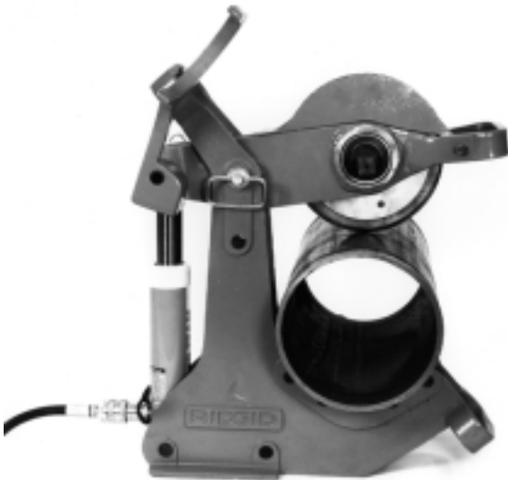
Figure 8 – Positioning Pipe in Cutter
