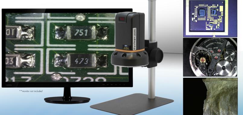
This innovative inspection scope connects directly to an HD monitor through a convenient 1080p HDMI output allowing operators to view high quality magnified images while looking straight ahead at a large screen, rather than hunching over narrow eyepieces. A large working distance and 30 LEDs that can be adjusted for intensity allow examination of objects of various sizes. Magnification ranges up to 132x on a 21.5" HD monitor.
