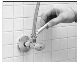
The open-end 12-point box line wrench is designed to slip over the supply tube and onto the riser nut. The 12-point box wrench allows you to grasp the riser nut in twice as many positions as a standard open-end wrench. No more "rolling" your wrench to get a grip.
