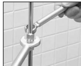
The insert in the larger wrench is made to grasp the narrow shoulder of the 3/8" coupling, or Delta Tube™. It holds the body in place while the 12-point line wrench tightens the 3/8" nuts.
