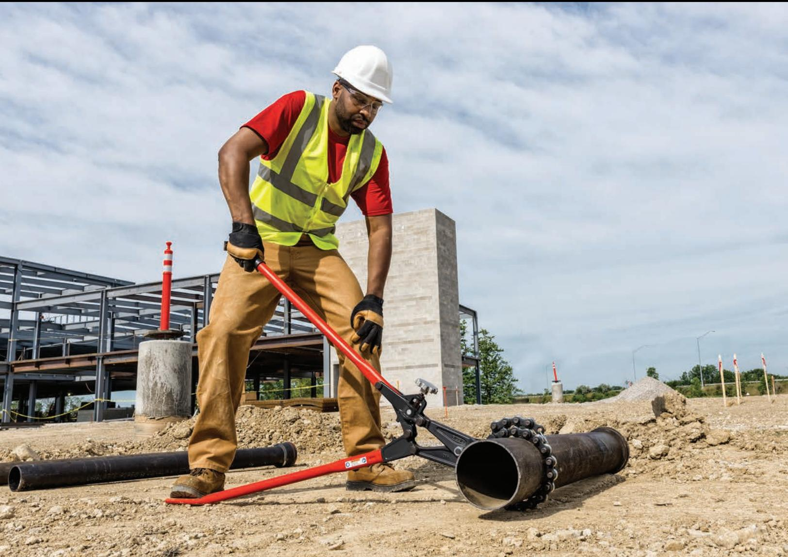
**Quickly make repeated cuts with a single stroke on soil pipe up to 6 inches.**
