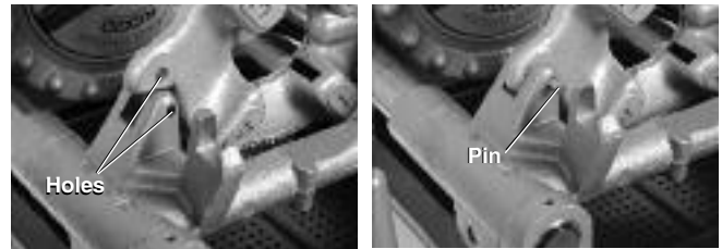
Figure 26 – Retaining LH Die Head in Place
