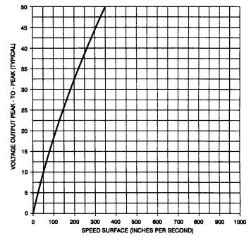
Shows peak-to-peak voltage output vs. surface speed of a 20-pitch, 30 tooth ferromagnetic gear at 0.005 inch clearance. Load = 100,000 ohms.
