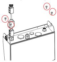
Install the indicator on the indicator support and tighten the handles at both ends, as the following step 1. Tighten the other end of the cable in the sealing kit and the connector on top of the sealing shell, as the following step 2. Finally, the entire sealed shell is hung in the two round holes at the upper end of the scale body as the following step 3.
