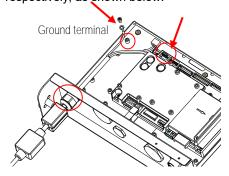
8. Pull in the bottom of the indicator. Re-install the 4 screws (Torque is 1.8N\*m±0.5). Fasten the cap nut of cable gland.
