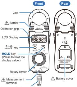
Test lead or flexible sensors plug
