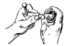
Maintain grip on jaws. Keep jaws in firm contact with body of wrench turning jaws 180°.
