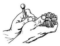
Spread jaws apart with thumb on side where ring is split. Slide jaws away from handle about 1/2 jaw length. It is not necessary to remove spring ring.
