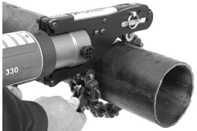
Figure 4 – Wrapping Chain Around Pipe
