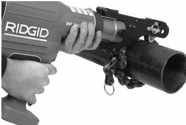
Figure 5 – Cutting The Pipe
