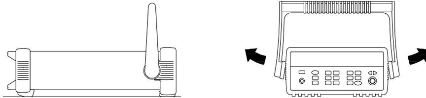
To remove the handle, rotate it to the vertical position and pull the ends outward.
