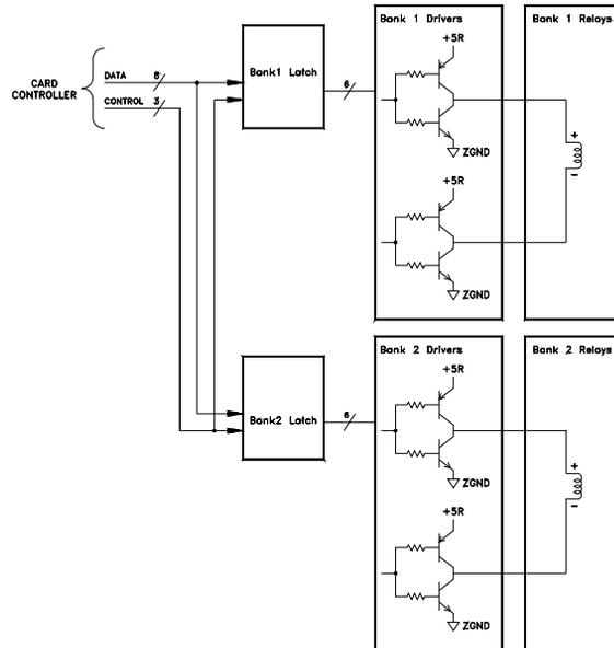
Bank1 latch, U102, and Bank2 latch, U103, control the relays. The bank drivers are divided into six groups of set and reset drivers. Each set and reset driver controls one relay. The column drivers operate as a pair. There are six column drivers each controlling a relay. The relays are arranged into two independent banks:
