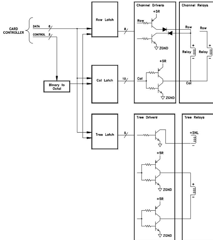
The row latch, U102, and column latches, U103 and U104, control the relays. The row drivers are divided into four groups of set and reset drivers. Each group of row drivers controls five relays. The column drivers operate as a pair. There are ten column drivers each controlling two relays. The analog bus backplane relays are non-latching.
