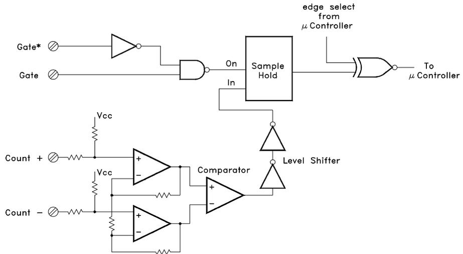
The totalizer counts signals connected to the COUNT+ and COUNT- inputs. Two op-amps, U108A and U108B, are used for input signal conditioning. Comparator U109 determines the signal trigger levels based upon the setting of the jumper at P102. With the P102 jumper in the TTL position, the totalizer counts pulses with TTL trigger levels. With the jumper at P102 in the AC position the trigger level is at zero.
