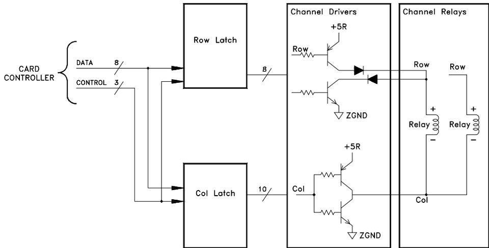
The row latch, U102, and column latches, U103 and U104, control the relays. The row drivers are divided into four groups of set and reset drivers. Each group of row drivers controls five relays. The column drivers operate as a pair. There are ten column drivers each controlling two relays.
