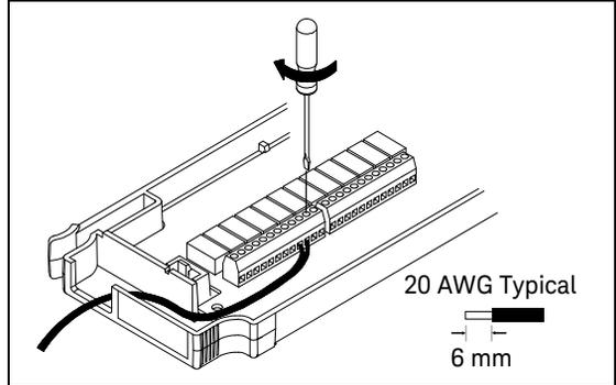
**3** Route wiring through strain relief.
