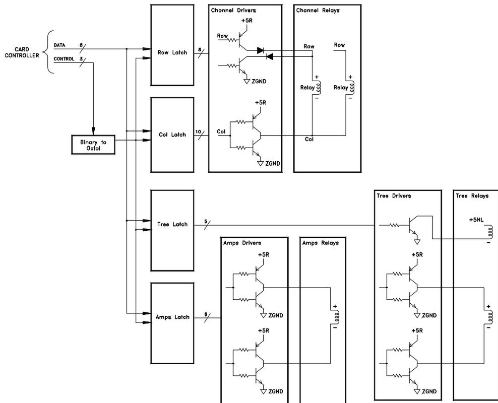
The row latch, U102, and column latches, U103 and U104, control the relays. The row drivers are divided into four groups of set and reset drivers. Each group of row drivers controls five relays. The column drivers operate as a pair. There are ten column drivers each controlling two relays. The analog bus backplane relays are non-latching.
