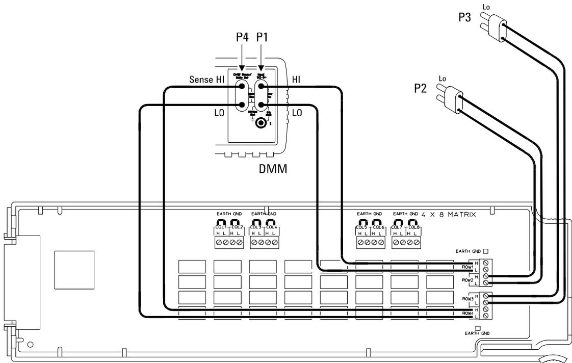
*Connections for 34904A Verification Tests*
