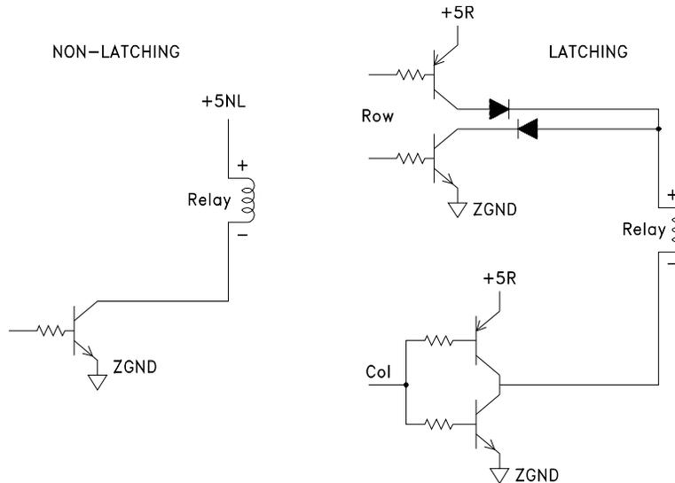
The non-latching relay contacts are in the set position (closed) when current flows through the coil. When the current is removed, the relay resets (opens). The positive side of the relay coil is connected to +5NL. The negative side of the relay coil is connected to ZGND through a single NPN transistor. The transistor and +5NL must be on for the relay to stay in the set position.
