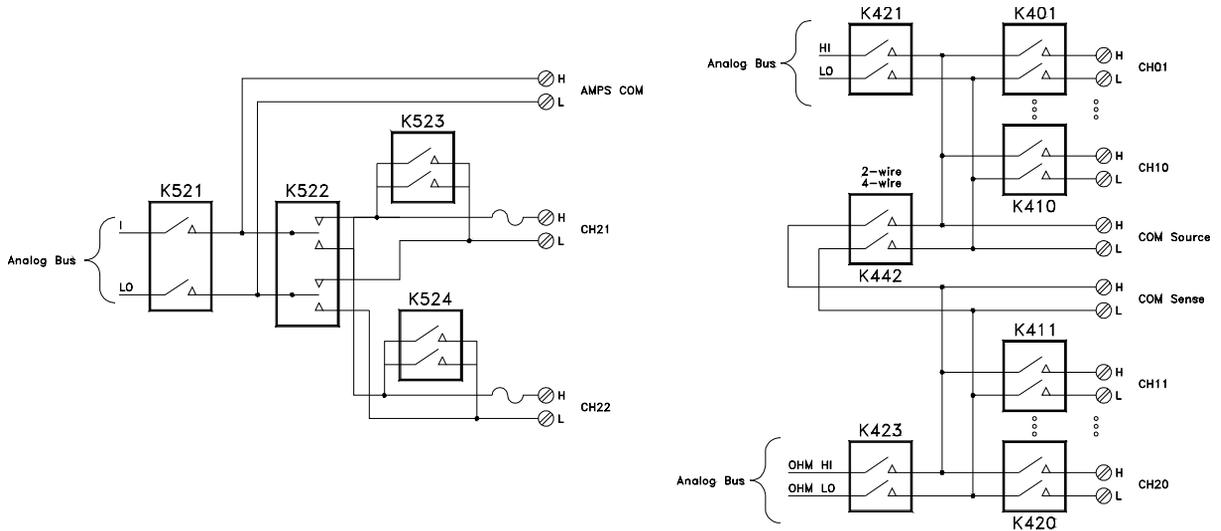
The current measurement channels are selected by relay K522. Relays K523 and K524 short the inputs when a channel is not selected. Relay K521 makes the connection to the analog bus for measurement by the Internal DMM.
