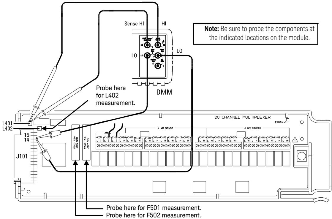
Connections for 34901A Verification Tests 1 through 5
