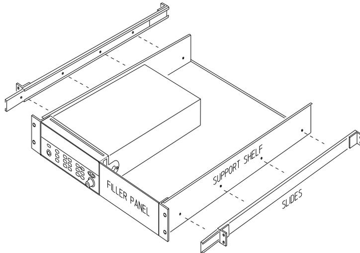
To install one or two instruments in a sliding support shelf, order shelf 5063-9255, and slide kit 1494-0015 (for a single instrument, also order filler panel 5002-3999).
