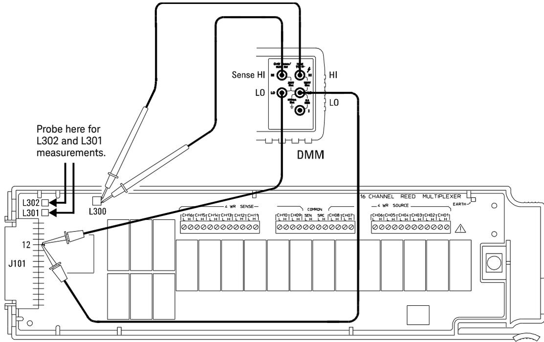
Connections for 34902A Verification Tests 1 through 4
