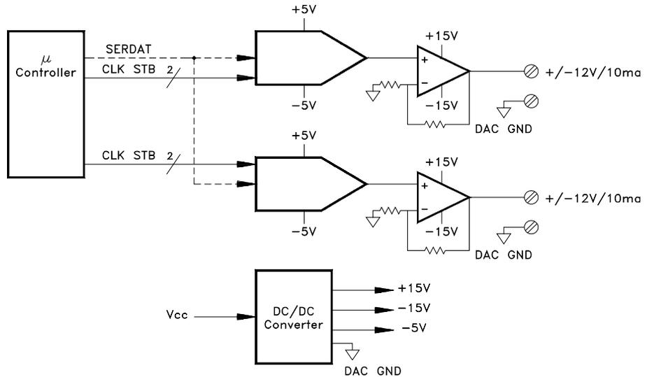
Communication with each DAC (U503 and U504) is via three lines: SERSTB, DACCLK, and SERDAT. Each DAC has a voltage output of  $\pm 3\text{ V}$ . U505 and U506 amplify this voltage to the  $\pm 12\text{V}$  output.
