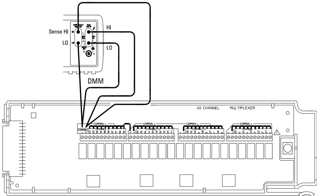
*Connections for 34908A Verification Tests 4 through 43*
