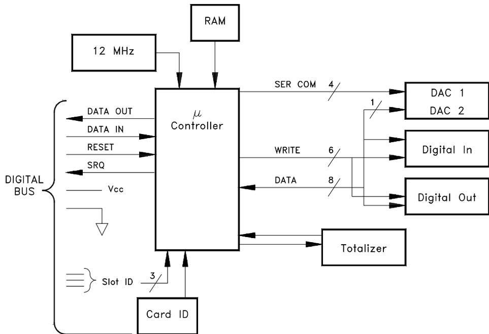
In addition to the +5 Volt power supply (Vcc) and ground, the module controller uses four lines for control and communication:
