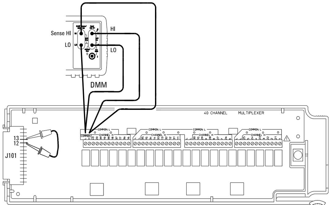
*Connections for 34908A Verification Tests 2 and 3*
