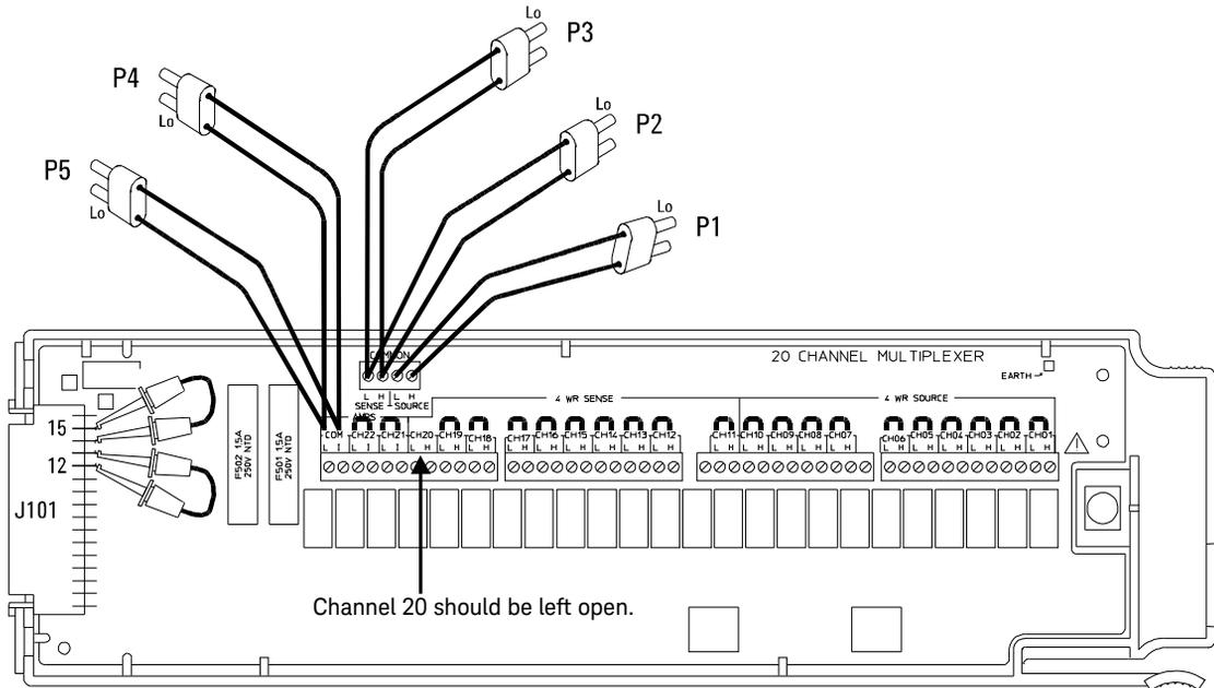
*Connections for 34901A Verification Tests 6 through 39*
