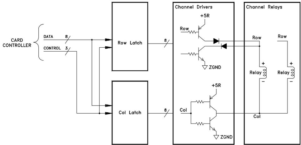
The row latch, U102, and column latch U103, control the relays. The row drivers are divided into four groups of set and reset drivers. Each group of row drivers controls eight relays. The column drivers operate as a pair. There are eight column drivers each controlling four relays. The relays are arranged in 4 rows by 8 columns.
