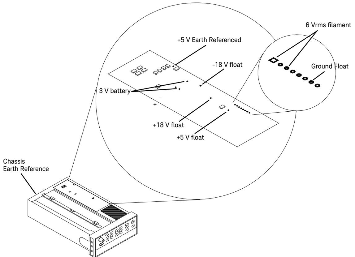
If you need to change the battery on the 34972A, be sure to unplug the instrument first. Use a CR2032 3V lithium battery, and insert the battery with the + side up. If you do not have a new battery, do not discard the old battery, as the instrument will not boot up without a battery - even a dead one - in place. Dispose of the old battery in accordance with local regulations.
