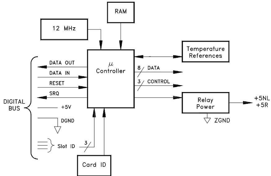
In addition to the +5 Volt power supply (Vcc) and ground, the module controller uses four lines for control and communication:
