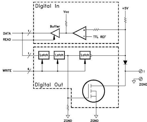
Two stages of latches on the outputs and one set of latches on the inputs provide synchronous 16 bit writes and reads of the digital ports.
