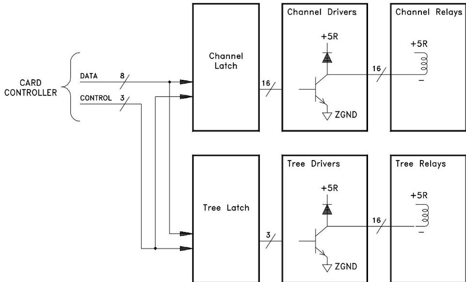
The reed relays are non-latching and the relay driver and +5R is applied while a channel is closed.
