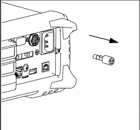
**2** Remove the fuse from the assembly.
