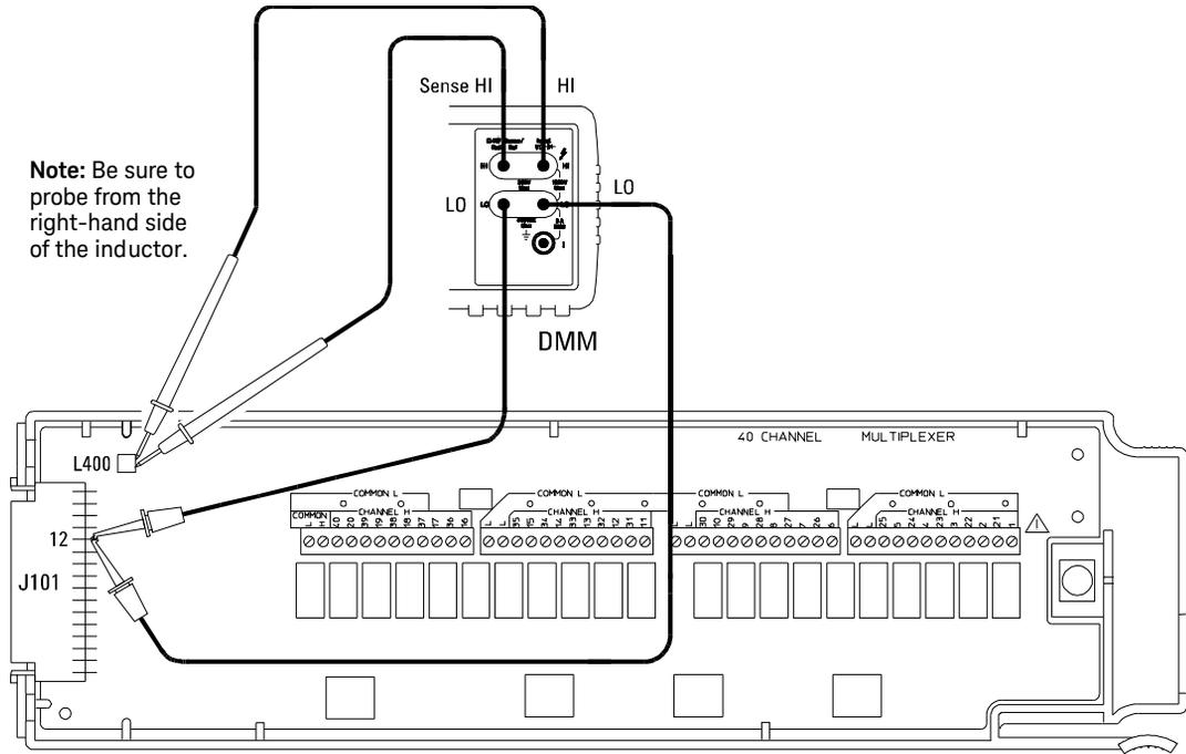
*Connections for 34908A Verification Test 1*
