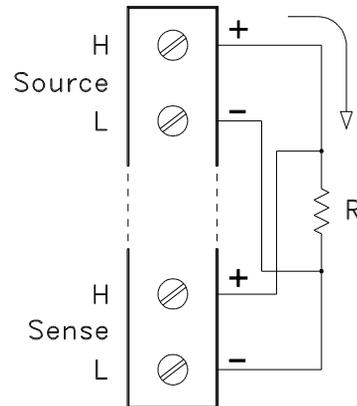
Channel  $n$  (source) is automatically paired with Channel  $n+10$  (sense) on the 34901A, or Channel  $n+8$  (sense) on the 34902A.
