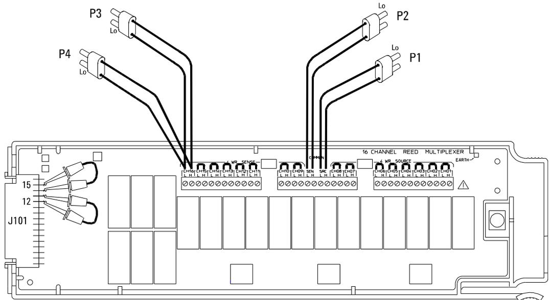
*Connections for 34902A Verification Tests 5 through 27*
