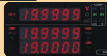
Voltage comparator setting
