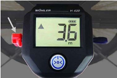
Fig. 23: Star grip screw for adjusting the freewheel brake
