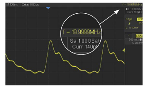
Built-in arbitrary waveform at 20 MHz, 300 MSa/s
