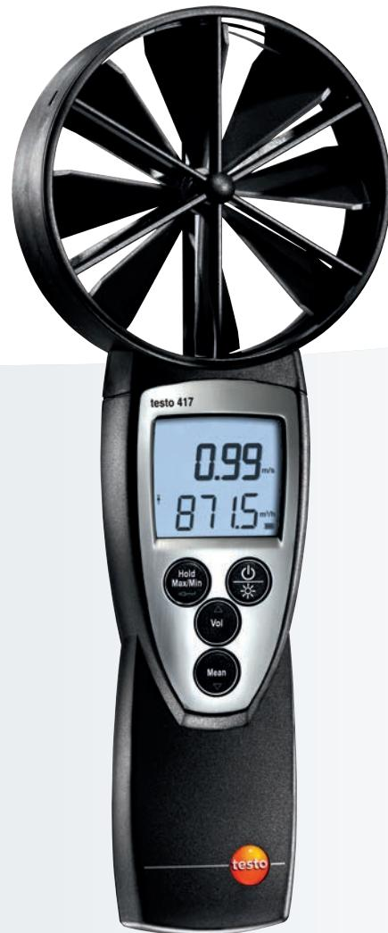
testo 417 is a compact, large-area anemometer with a built-in flow velocity / temperature vane. It measures flow velocity, volume flow and temperature. Thanks to the integrated measurement with the 100 mm vane, it is ideally suited for measurements at air input and output vents. The flow direction, i.e. blowing or sucking flow, is visible in the display. The optimum funnel set additionally allows measurements on ventilation grilles and disc outlets.
