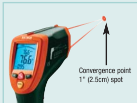
Two laser points converge at a distance of 50"/(127cm) and form a 1" (2.5cm) spot.
