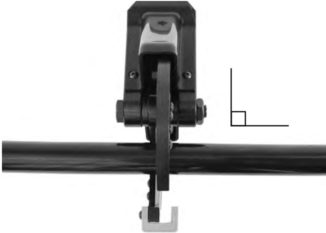
Figure 3 – Cutter Square to Wire
