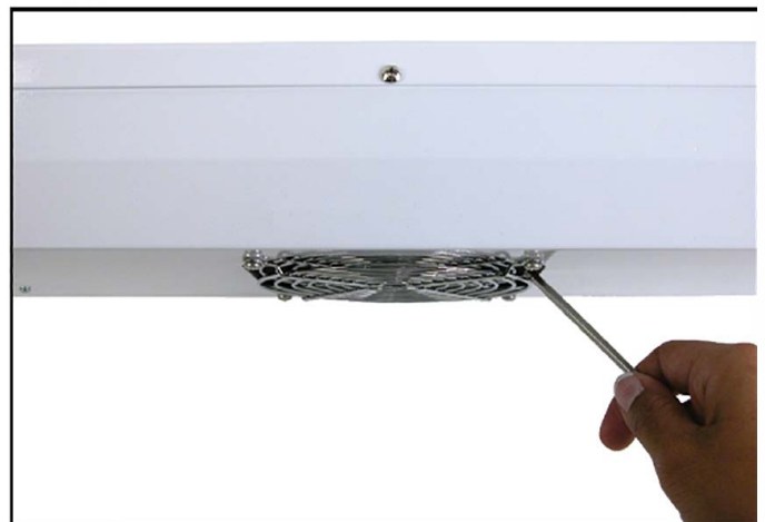
Figure 10. Shorting the ionizer's two fan grills
