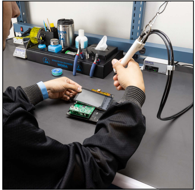
Figure 7. Using the Pencil Type Ionizer
