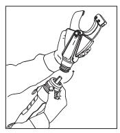
Remove the head by pulling the movable collar toward the base of the tool.
